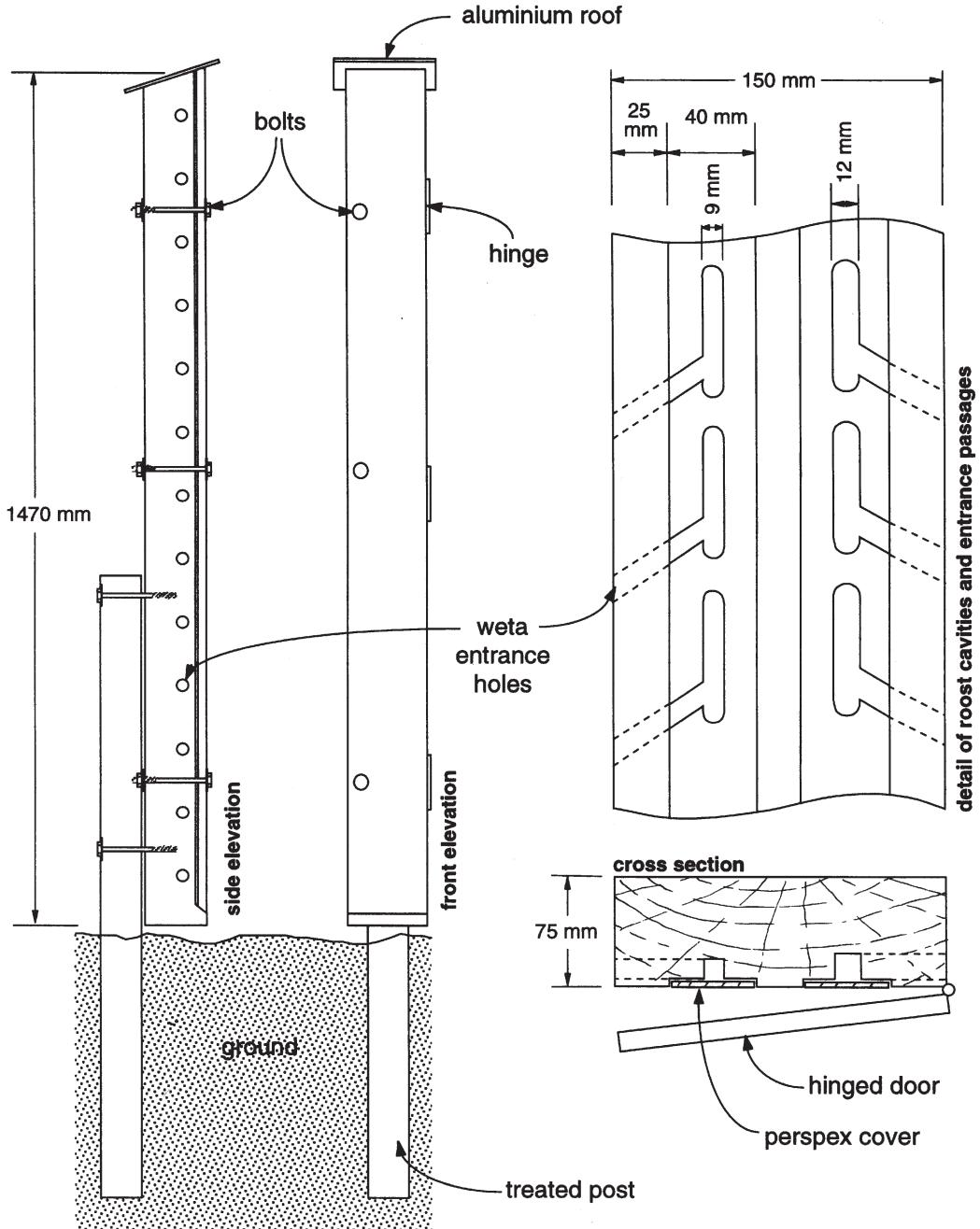
Figure 1. Design of original weta roosts deployed at Mohi Bush in 1994.
